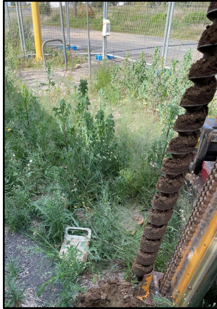
Figure 14. Drilling of S3. The soil is Dark Grey Medium Clay within fill layer.
